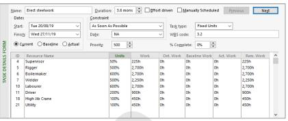
The duration has extended to 3.6 months because the Work for the Riggers (2,700h) is now divided by 5 riggers to derive total work of 540 hours for each rigger. Since there are 150 hours of work per week (37.5 x 5) when you divide the total hours (540h) for a rigger by 150 you get 3.6 months.
