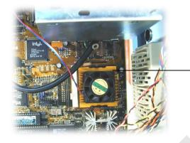
The CPU chip inside a personal computer is sometimes a bit tricky to spot. It is large and often has its own cooling fan sitting on top.
