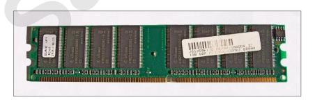
So RAM is volatile, meaning that its contents will be lost as soon as there is an interruption to power. RAM is also constantly changing with new contents flowing through on a regular basis.
